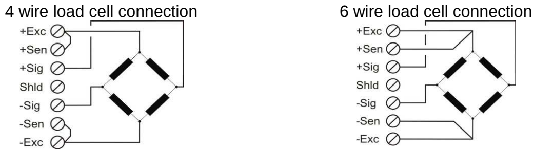
Figure 6.3 - Load cell connection
